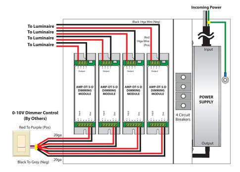
**ADNM-240-3-5-12-DOT** 120-277V AC / 12V DC, 180W /3 CIRCUITS X 5A **ADNM-320-3-4-24-DOT** 120-277V AC / 24V DC, 288W /3 CIRCUITS X 4A
